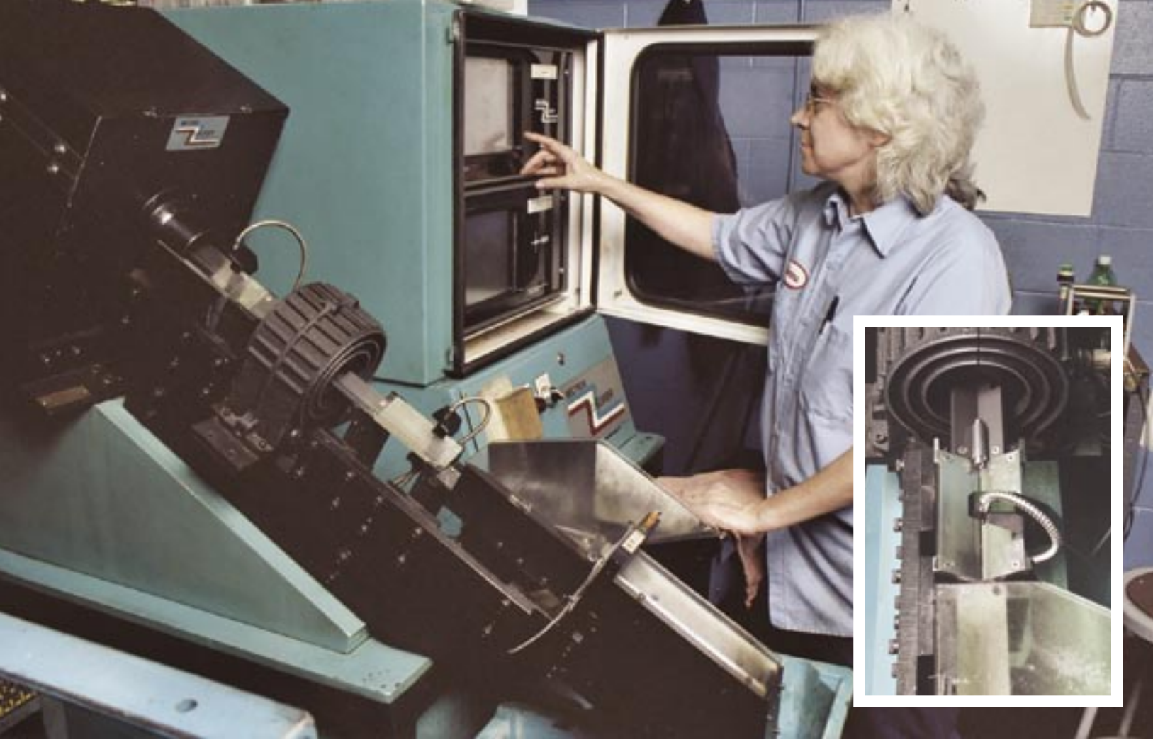
Operator Glenna Kindle checks the status of parts running (see inset) through BMC's Mectron inspection unit. The machine's high-speed capacity allows for faster sorting and defect identification on large volumes of parts, helping meet ever-increasing quality demands from customers.
